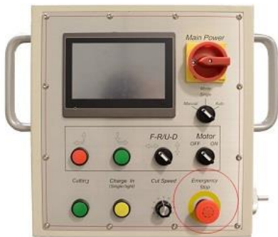
Emergency Stop Button
