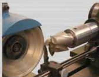
Optional Extension Bushing for tools with 1 1/4, 1 1/2, 2" diameter shanks
